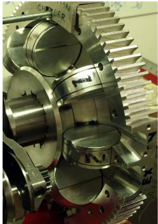
Piston Closeup: Eight pistons on two shafts give the MYT engine 850cu of displacement.
