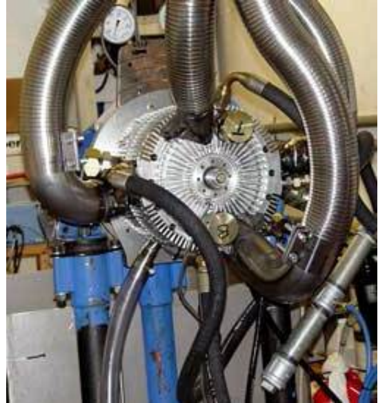
Air Motoring: Compressed air testing at 150 psi generates over 800 ft/lbs of torque!
